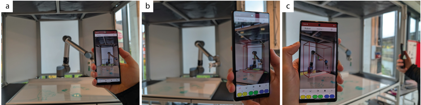
Figure 1: Exemplary use of the DangAR application in a human-robot collaboration context: a) The user can place a danger zone freely around the robot, b) transform it to the desired location, and c) collaborate with other domain experts in real-time to fine-tune the danger zone spatial configuration.
