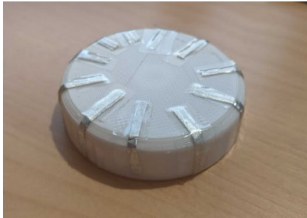
Figure 1: First Prototype: Using conductive ink on an existing USB knob.
