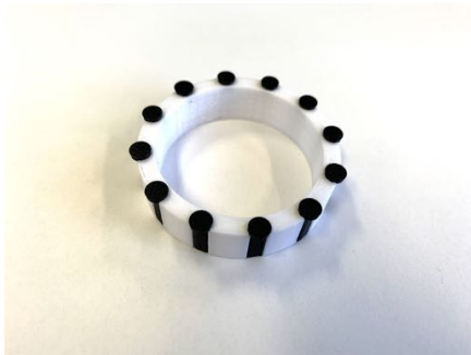
Figure 3: Second Prototype: Final iteration using conductive filament.
