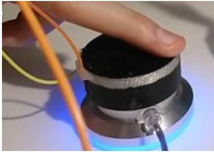
Figure 1: First Prototype: Using conductive ink on an existing USB knob.
